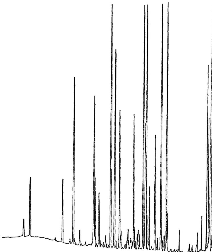
Fig. 5. Chromatogram of a Bouquette essential oil sample (batch No. 6716). Carrier gas, nitrogen; initial temperature 50°C; programming rate, 3°C/min; final temperature, 240°C; column, 40 m  $\times$  0.37 mm I.D. BaCO<sub>3</sub>-treated Pyrex capillary coated with 0.25- $\mu$ m Pluronic F68; sample volume injected, 1  $\mu$ l; splitting ratio, 1:50.
