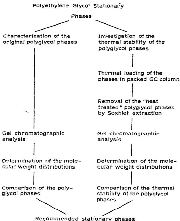
Fig. 1. Schematic diagram of the experimental procedure.
